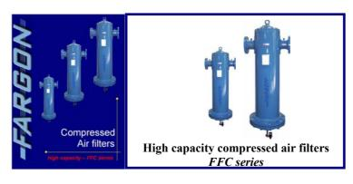
Complete line of purifiers filters for air - high capacity (flow rates up to 22,000 Nm³/h or more on request - pleated, sintered, coalescing and activated carbon - up to 10 bar pressure or larger upon request)
