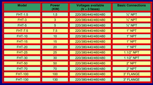
note: the basic connections may change depending on the flow and temperature of heating required.
