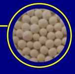
Some compressed air applications requests a low moisture level (dew point between -5 to  $-70^{\circ}$ C), not being attended by the conventional refrigeration air dryer systems (dew point +3°C). In this case we must use the dryer that operates by adsorption process.
